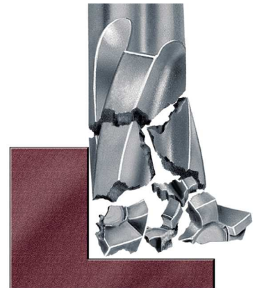
CRACKED SOLID CARBIDE TOOL SHATTERS
